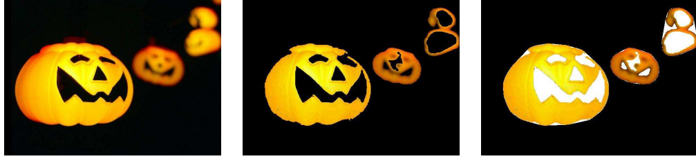
Figure 5.13. Demonstrating the shape convexity feature. Left: Original photograph. Middle: Three largest non-background segments shown in original color. Right: Exclusive regions of the convex hull generated for each segment are shown in white. The proportion of white regions determine the convexity value.
