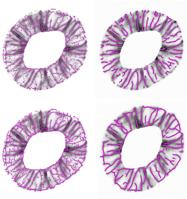
Figure 6.1: Improvements benefiting from a heuristic initialization. The second column shows seed points through tangential local maxima as opposed to ridge detection in the first row.
