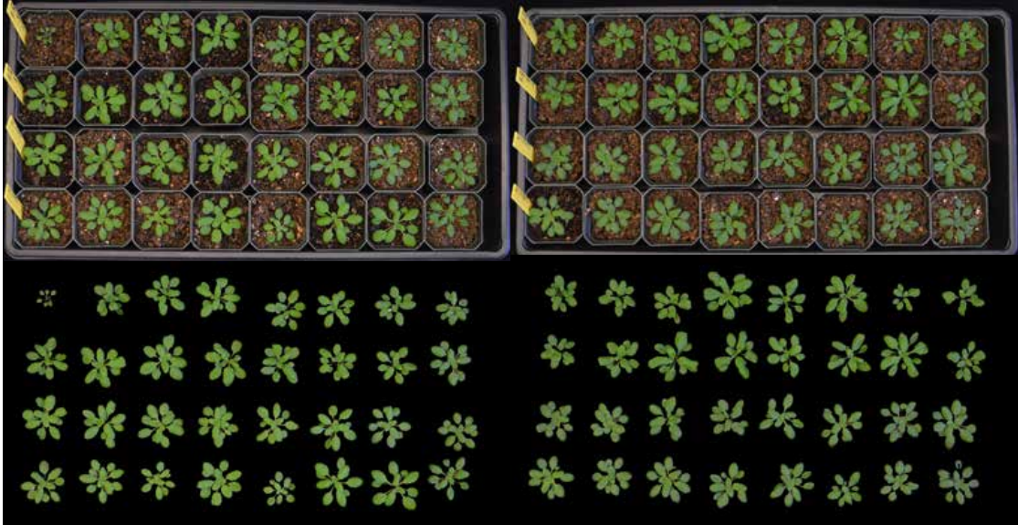
Figure A.1: The segmentation of leaves by thresholding according to their hue, saturation and value(brightness).
