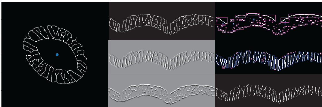
Figure 6.4: The artifact removal problem becomes easier as the resulting snakes are converted to polar coordinates. The boundary artifacts and tubules separate into vertical and horizontal structures. The use of a Sobel edge filter applied to the binary image can delineate these structures. The bounding box of connected components provides an idea of the structure orientation. The magenta bounding boxes show horizontal structures in both of the thresholded horizontal and vertical difference images.
