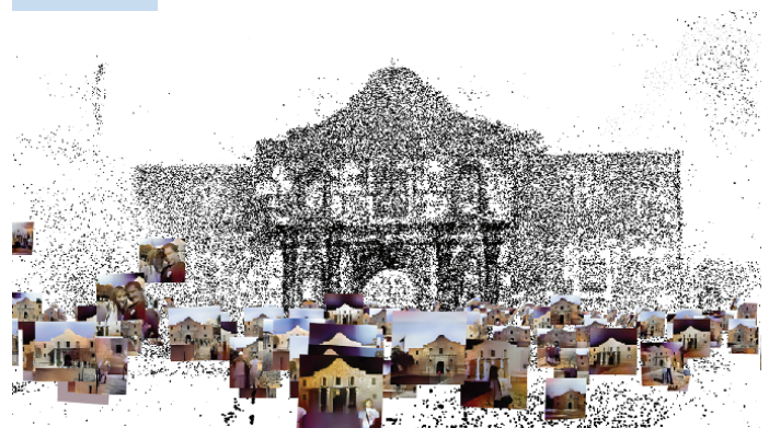
Image reconstructions, displayed with their estimated poses and the triangulated point cloud.
