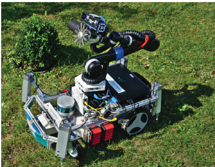
The TrimBot2020 gardening robot, with the topiary trimming end effector
