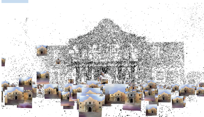
Image reconstructions, displayed with their estimated poses and the triangulated point cloud.
